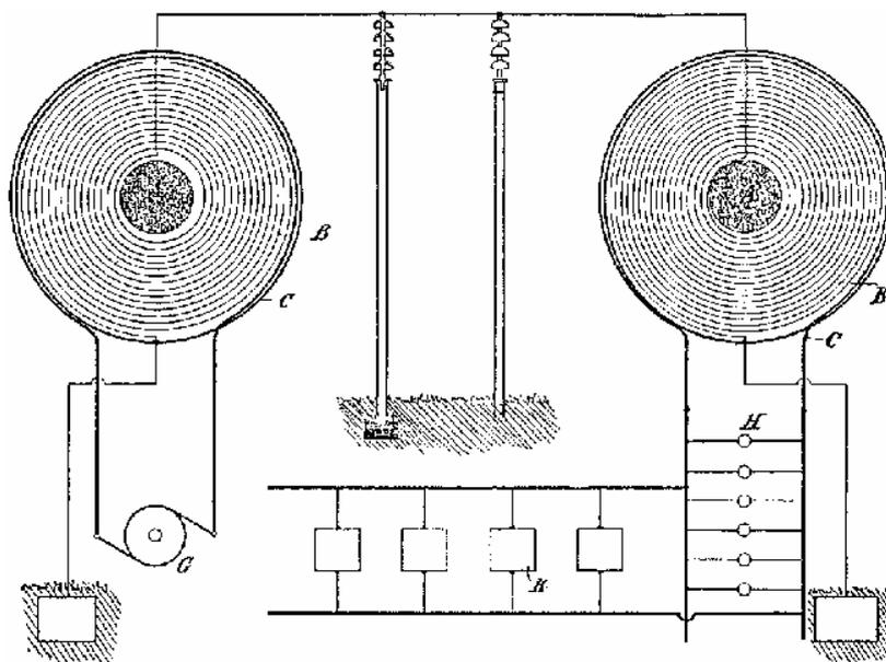
Figure 2: US-Patent 593,138 „Electrical Transformer“ issued on November 2<sup>nd</sup>, 1897
