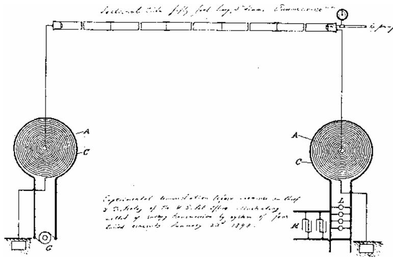
Figure 3: Slide of Nikola TESLA<sup>[27]</sup> about the energy transmission through a partly evacuated glass tube; dated of January 23<sup>rd</sup> 1898.
